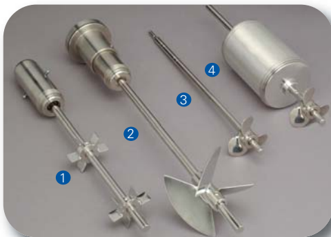
Four impeller options provide flexibility to grow a wide variety of cell lines. Choose: 1. Rushton impeller for standard fermentation applications. 2. Low-shear Pitched blade or 3. Marine blade impellers for gentle mixing of shear-sensitive cell lines such as insect, plant and animal cultures. 4. Spin filter — a cell-retention device used with a marine blade impeller — for perfusion processes using anchorage-dependent or suspension cultures.
